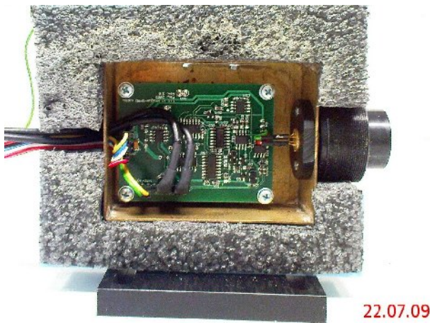
Fig. 3. The laboratory sample of the photon counting detector package for the ELT mission, version 3.0 installed in the temperature control box. The active quenching and gating circuit is based on fast PECL circuits, the K14 detection chip (right).
